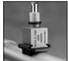
Fig. 6 The Mounting Clip with Thick Base UA 1475 can be filed down to suit your mounting surface needs. Here it is mounted on a tube with Type 4508
