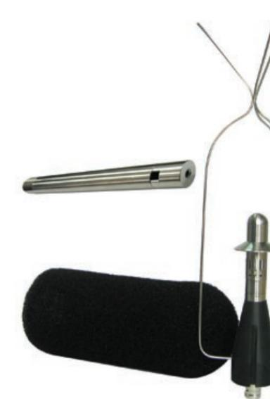
**OM231** is 1/2 inch prepolarized condenser outdoor microphone. It is suitable for use in rainy days or in an environment at very high or very low temperature. OM231 uses IEC 61672 CLASS 1 measurement microphone which is outstanding for its stability. It is the best choice for permanent outdoor use such as the airport noise monitoring.
